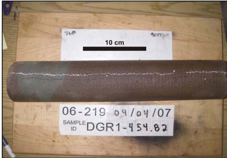
Figure 5.5.2-2: Core Sample of Green and Red Calcareous Shale, Upper Ordovician Queenston Formation, 454.82 mBGS, DGR-1
